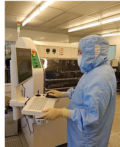
Class 100 clean room automated die attach
